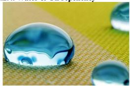
Water and Oil repellency happens when the surface tension of the solid surface is lower than that of oil & water. As such water and oil will enter the fabric surface as surface tension of cotton is higher than that of Oil & water. When the fabric is treated with this finish the surface tension is lowered than that of the Liquids. Hence your garment becomes Water and Oil Repellent.
