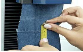
In some garments seams slip at the slightest force applied. This can be corrected by using a special auxiliary. In addition to preventing seam slippage, the strength is also increased by this treatment.
