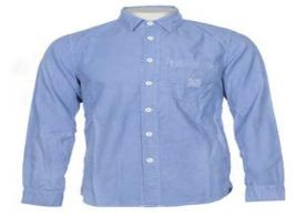
Delicate light weight garments which require the stone wash effect are washed with perlite powder in place of Pumice stones to avoid damage. The advantage is that we get the stone washed effect throughout the fabric and not just on the upper surface as in case of stones.
