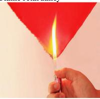
Flame retardants improve the resistance to ignition of the Substrate thereby reducing the chance of starting a fire. In case of a fire they reduce the flame spread and rate of fire development, thus providing extra time to extinguish the fire or make an escape. Flame retardants act physically as well as chemically in combating the fire by cooling the substrate, forming a protective layer over it, diluting the combustible material and also by chemical reactions.
