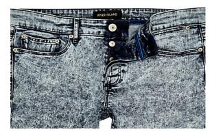
This term is a complete misnomer as virtually no acid is used in this process. Denims are washed with pumice stones soaked with hypo to give significant contrast in the color of the Denim Material. The same process can be employed on yarn dyed garments giving several finishes. In this process pumice stones are substituted with thermocol balls.
