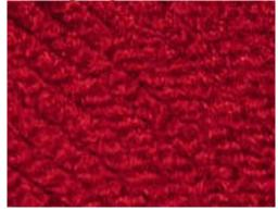
This treatment reduces the forming of pills on fabrics and knitted products made from yarns with a synthetic fibre content, which are inclined to pilling by their considerable strength, flexibility, resistance to impact. This finish is based on the use of chemical treatments which aim to suppress the ability of fibres to slacken and also reduce the mechanical resistance of the synthetic fibre.
